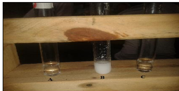
Fig. 5. Image of the distillate test. Laboratory Distilled Water (A), Sol. Sodium Chloride (B) and Water from the homemade distiller (C).
